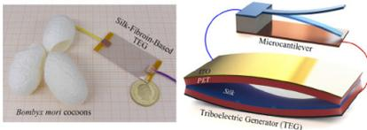
Fig. 1 Photograph of the silk-based triboelectric generator (TEG) and schematic view of driving a microscale cantilever by using the fabricated TEG.
