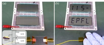
Fig.2 Two 4-bit liquid crystal displays were successfully directly driven by the fabricated triboelectric generator (TEG) without any external circuit.
