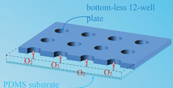
Figure 1 : Bottom-less 12-well plates fixed on PDMS substrate
