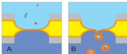
Fig. 1. Formation scheme: A) a bilayer formed in a planar nozzle between two water phases supported by an infinite phospholipid-in-oil reservoir. B) Deformation of the bilayer, enveloping the disperse phase (above) while continuously separating the continuous phase (below).
