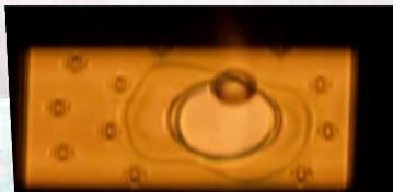
Fig. 2. Bottom-up view of the injection of a femtoliter oil droplet in the water reservoir through the planar nozzle. The device is about 200  $\mu\text{m}$  long
