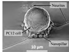
Fig. 1. Scanning electron micrograph of a neuron on a nanopillar array with neurite growth
