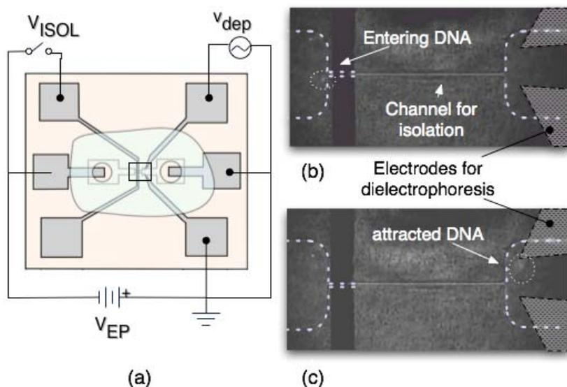
Figure 2 : Microfluidic chip (a) schematic of the chip with inlet/outlet and bias. Enlarged view of the chip center with (b) DNA entering in the channel and then (c) attracted by DEP.
