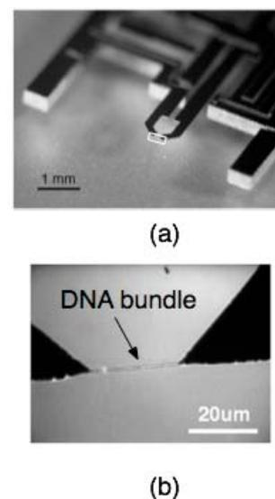
Figure 3 : tweezer. (a) processed device. (b) trapped DNA bundle.
