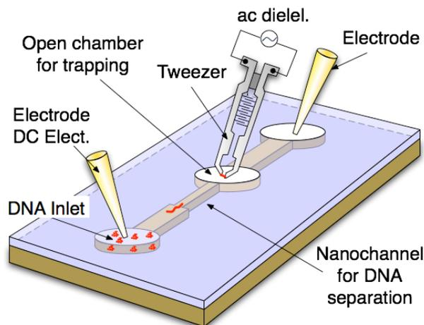
Figure 1: Molecule isolation and trapping
