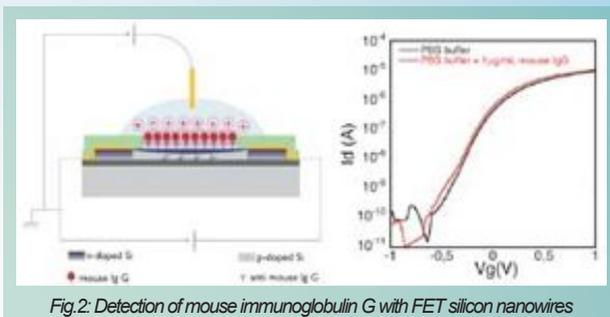
Fig.2: Detection of mouse immunoglobulin G with FET silicon nanowires
