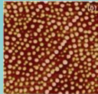
Fig. 1:  $1 \times 1 \mu\text{m}^2$  AFM image of uncapped InAs QDs grown on GaAs/GeOI substrate
