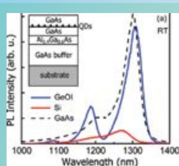
Fig. 2: RT PL spectra of the InAs QD samples grown on silicon (red curve), GaAs (dashed curve), and GeOI substrate
